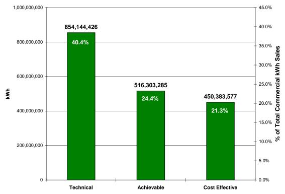
Table 6-5 and Figure 6-4 show the total achievable cost effective potential kWh savings for existing commercial buildings within each of the commercial end uses. Lighting accounts for the largest percentage of savings potential at 41 percent, with refrigeration being the second largest at 36 percent. Space cooling and related HVAC controls are third largest at 13 percent and water heating, space heating, motors, and miscellaneous loads represent the remaining 10 percent.
