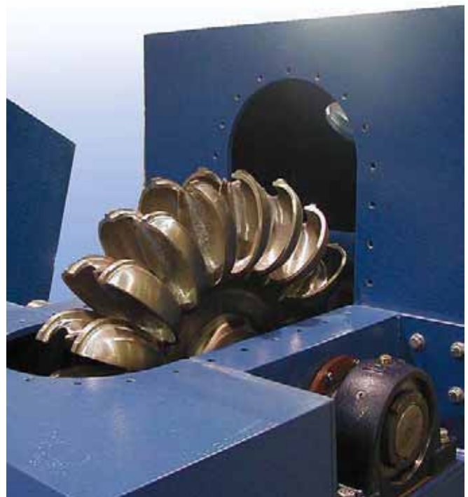
A view into a turbine shows a relatively large (2 feet in diameter) Pelton wheel. Peltons vary in size from 3 inches to 13 feet or more, depending on head and flow.
