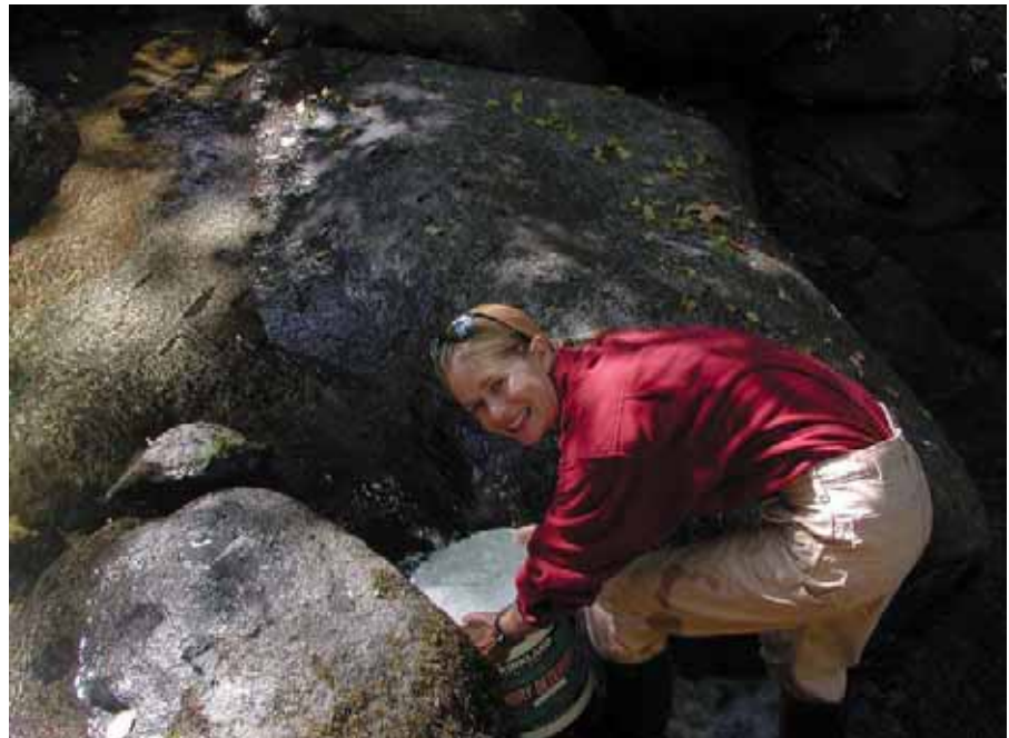
Anna gets her feet wet—the container fill method of measuring flow means getting in the stream and timing how long it takes to fill a container of known volume.
