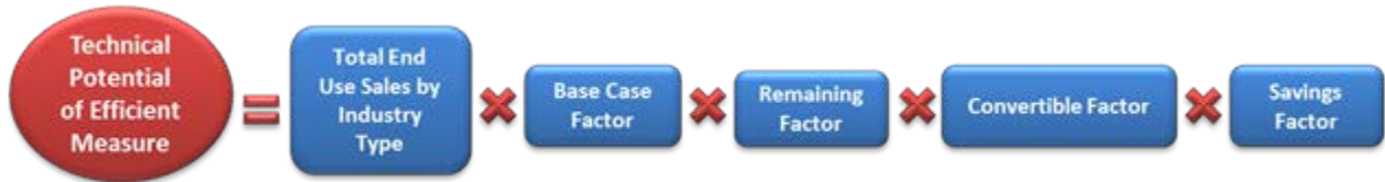
Equation 4-1: Core Equation for Non-Residential Sector Technical Potential
