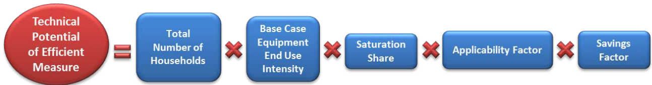
Equation 3-1: Core Equation for Residential Sector Technical Potential
