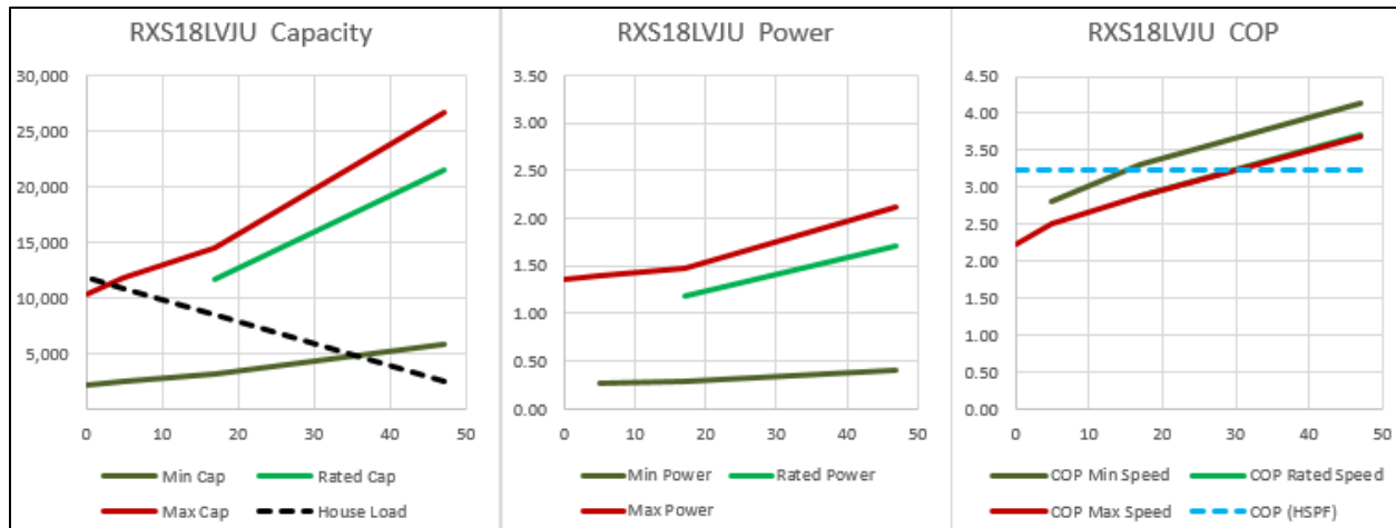
Figure 4. Example of Manufacturer's Information for Daikin Cold Climate Heat Pump
