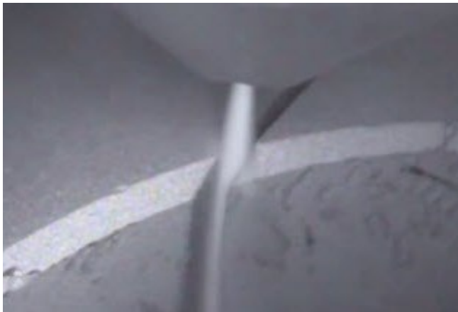
Abrasive water jet slicing metal part
